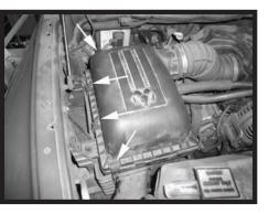
Step 3 Unclip the four hold down clips on the air filter lid.
