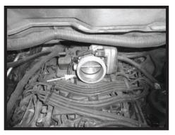
Step 6 Remove the o-ring surrounding the throttle body.
