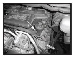
Step 2 Disconnect the factory PCV breather hose from the engine.
